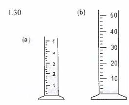
The 5 mL graduated cylinder is marked every 0.2 mL and can be read to  $\pm$  0.02 mL. The 50 mL graduated cylinder is marked every 2 mL and can only be read to  $\pm$  0.2 mL. The 5 mL graduated cylinder will give more accurate measurements.
